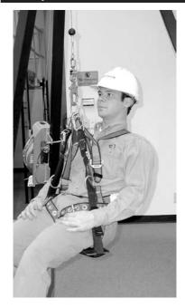
The primary function of the MSA Bosun Chair is to serve as a work positioning device. It provides comfort by relieving pressure on the sub pelvic area of the user and his or her full body harness. The Bosun Chair is not intended nor is it designed to be used without other fall protection equipment.
