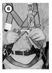
**7.** Attach the chest D-ring to the lifeline connector, i.e. - winch, descent control device or other raising, lowering device.
