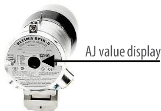
Figure 8: Receiver unit with built-in alignment indicator
