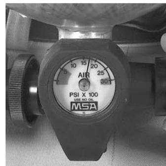
4. As the pressure rises from 50 to 200 psig, the alarm sounds automatically, indicating that the alarm is functional.
