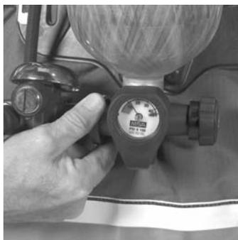
3. Check that the cylinder is fully pressurized.
