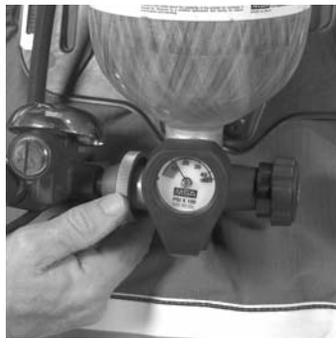
2. Lift and turn the latch wing to loosen the cylinder clamp.
