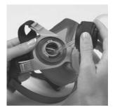
b. Pull the tube through and attach the adapter to the bayonet fitting on the respirator (as though installing a cartridge or filter). Use a clockwise motion and ensure the bayonet flanges are properly aligned. There are two larger flanges and one smaller flange.
