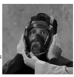
**Note:** To perform the negative pressure seal test, the inhalation port side of the Advantage Fit Test Adapter will need to be covered. This can be done with the help of the person assisting with the fit test.
