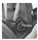
b. Pull the tube through and attach the adapter to the bayonet fitting on the respirator (as though installing a cartridge or filter). Use a clockwise motion and ensure the bayonet flanges are properly aligned. There are two larger flanges and one smaller flange.
