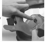
e. Don the facepiece and perform a negative pressure test by placing a finger over the end of the tubing connector and following negative pressure test in the respirator user's instructions manual.
