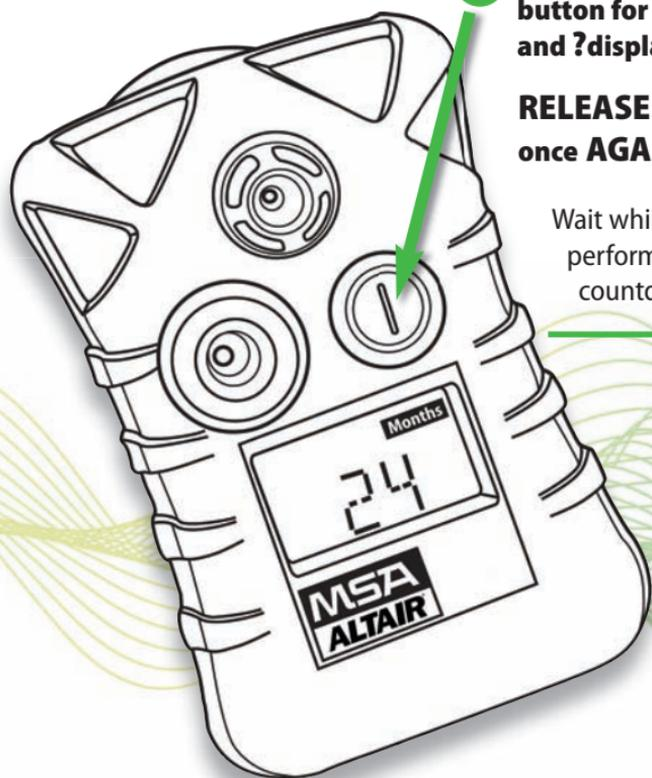
**2** **PRESS and HOLD** the **TEST** button for **5 seconds** until **ON** and **?display**.
