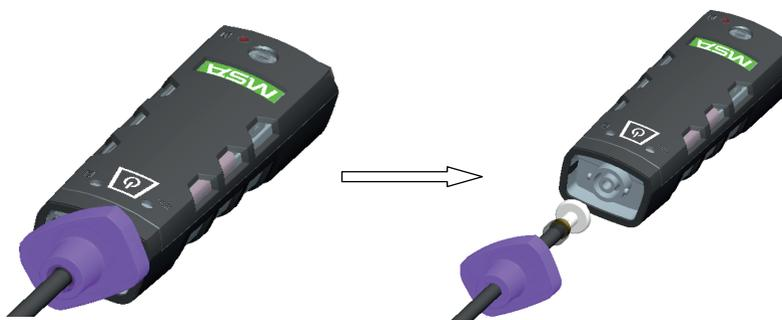
Fig. 3 Replacing Probe Filter
