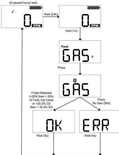
**Fig. 6 Conducting the bump-test**
