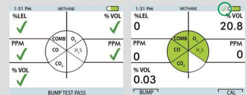
After BUMP TEST PASS appears, detach the cylinder. (If there are more sensors to be bump tested, the next sensor displays and the process repeats.) Cancel occasionally occurring alarms by pressing the **UP** button and check if the **✓** is displayed. (YES = ready for use, NO = repeat Bump Test) Record the results.
