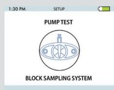
Block sampling system (pump inlet or sampling line) until PASS message appears.
