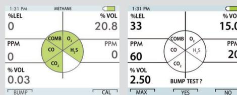
Select BUMP in the MEASURE page by pressing the **DOWN** button, press **ON/OFF** (YES) button to perform Bump Test, connect the correct calibration gas cylinder with your device and wait.
