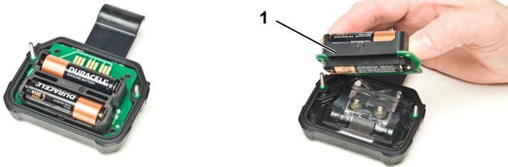
**Figure 4-3 Battery Replacement**
