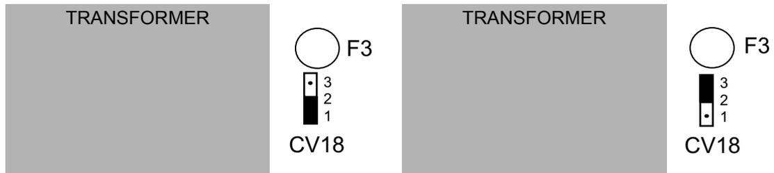
Fig. 10 24 VDC Power Supply from internal source Fig. 11 24 VDC Power Supply from external source
