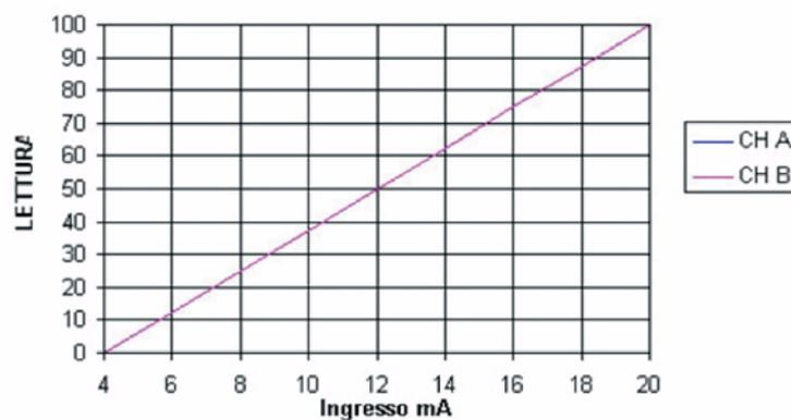
Fig. 13 Response curve for mA input
