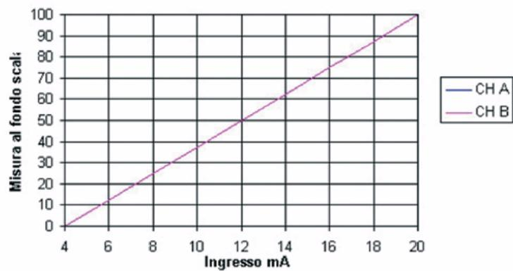
Fig. 14 Response curve for mA input
