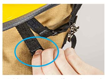
**4.** For helmets equipped with optional four-point chin strap, with main chin strap connected and cinched, pull additional straps and connect hook to loop. As with others, this adjustment should be made to maximize helmet fit, stability and comfort.
