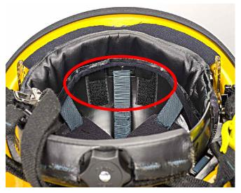
**1.** Adjust front headband ride height by pulling Velcro tabs apart; set height to a position that maximizes helmet fit, stability and comfort.
