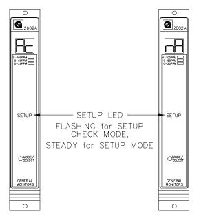
Figure 32: Alarm Output Option During a Card Test, AC/nA
