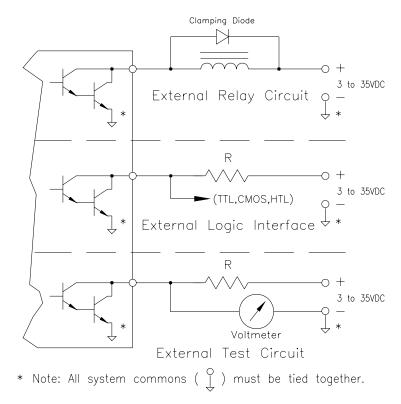
Figure 6: Typical External Circuits for Open Collectors
