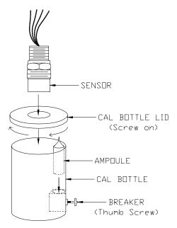
Figure 12: Breaker Bottle Operation
