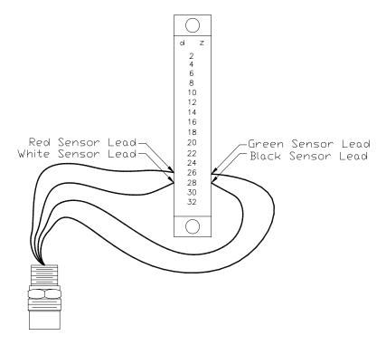
Figure 7: Sensor/Controller Connections
