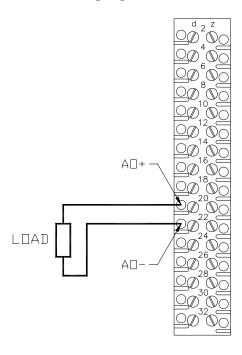
The maximum load resistance between  $A\Box + \& A\Box - cannot exceed 500 ohms.$
