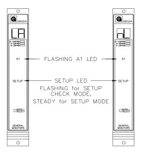
Figure 27: A1 Latching/Non-Latching Alarm Option
