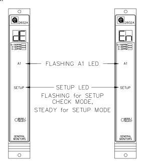
Figure 26: A1 Energized/De-Energized Alarm Option
