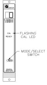
Figure 13: Entering the CAL Check Mode
