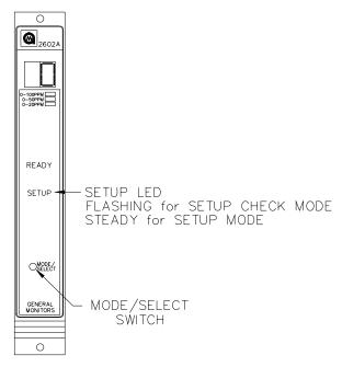
Figure 20: Entering the Setup & Setup Check Modes
