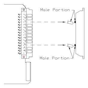
Figure 2: Control Module Coding Strip
