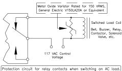
Figure 5: Protection Circuit for Relay Contacts
