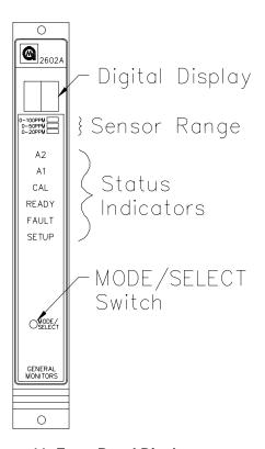
Figure 11: Front Panel Display
