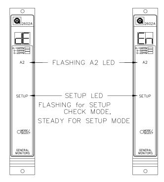
Figure 23: A2 Energized/De-Energized Alarm Option
