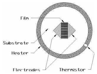
Figure 35: MOS Sensor Diagram, Top View
