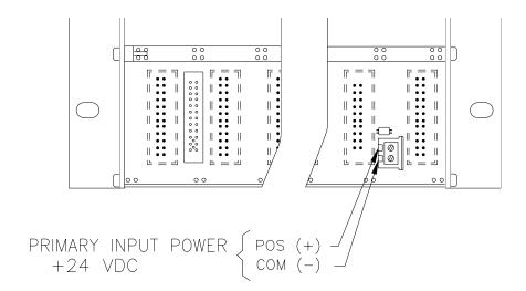
Figure 10: Power Connections for Rear Chassis
