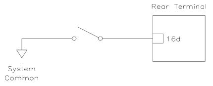
Figure 8: Card Test Switch Wiring
