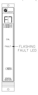
Figure 19: F7 Display During Cal Mode
