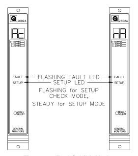
Figure 29: Fault/Inhibit Mode
