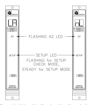
Figure 24: A2 Latching/Non-Latching Alarm Options
