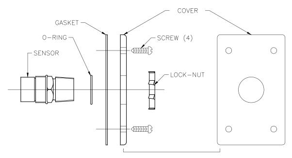
Figure 41: Duct Mounting Plate
