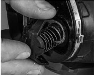
13. Install the spring retainer over the boss of the exhalation valve. Make sure the spring is seated correctly.
