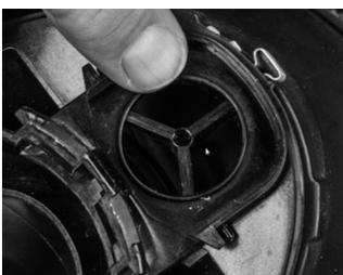
8. Use a wipe dampened with isopropyl alcohol to clean the surfaces of the valve seat.
