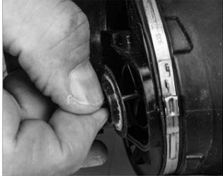
12. Install the new exhalation valve into the component housing. Make sure the valve stem is inserted into the stem opening.
