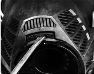
1. Insert a small flat-blade screwdriver into the tabbed slot below the lower button of the component housing.
