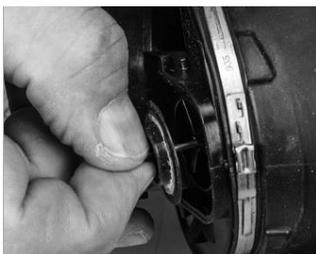
7. Remove the exhalation valve from the housing assembly, and discard it.
