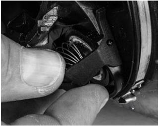
14. Align the retainer forks on the flat surface of the component housing, and slide the spring retainer forward until each fork snaps into position.
