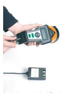
Charging is in progress when the red LED on the charger is lit.
