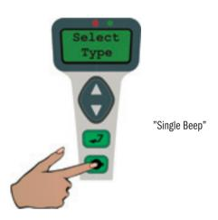
To power off the Gassonic 1701, hold down the button for approximately 3 seconds:
