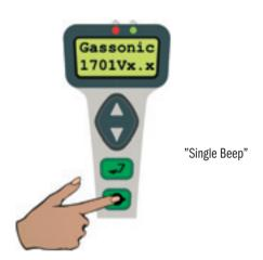
To switch on the backlight in the display and the flash light at the front end of the unit:
