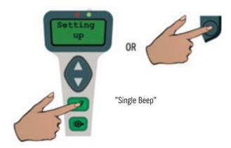
The Gain Test is done automatically while "wait..." is displayed. Pressing one of the two buttons again will abort the test.
