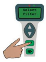
Select the correct filter setting (corresponding to the internal filter setting on the Gassonic MM0100, which is factory set to 25kHz).
