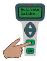
Set the Gassonic Observer into Calibration Mode (see Installation and User Guide), turn and lock the Gassonic 1701 over the sensor-head of the Gassonic Observer.
