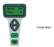
Another gain test can be performed immediately, on the same or another detector, by simply starting the test again.
