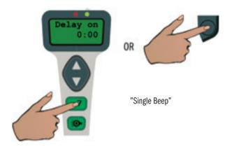
The actual test time elapsed is shown on the display. When the control room observes an alarm, press "ENTER" or "TEST" to stop the test. The time readout on the display corresponds to the alarm delay setting of the system. This delay should be at least 10 seconds.
