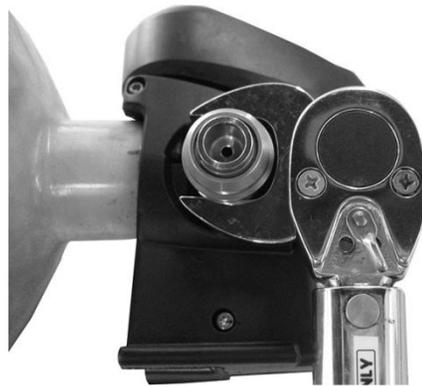
Upon installation of replacement quick connect adapters, it is important to discard the old adapters so they are not reused.
