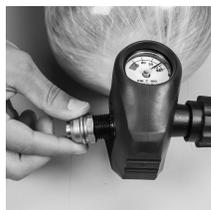
**NOTE:** A calibrated torque wrench with 24 mm open end Crowsfoot is required for installation.
