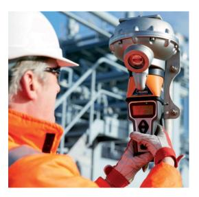
Although the GASSONIC detectors do not require regular maintenance, the GASSONIC 1701 can be used to satisfy the requirements for regular plant maintenance. Compared to traditional detection methods, calibration gas is not needed for testing the functionality of
