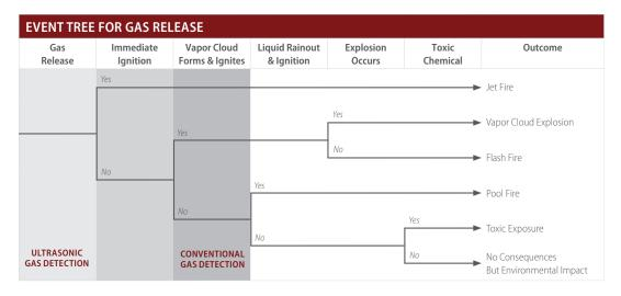
The gas release event tree illustrates the sequence of events that can take place in the event of a gas release. The figure shows that UGLD responds at gas leak initiation whereas conventional detectors only respond when the gas has accumulated and formed a vapor cloud.
