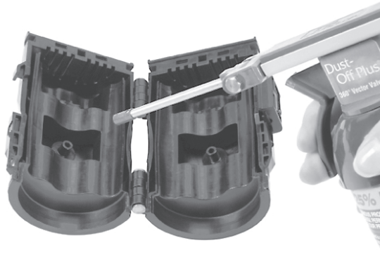
Fig. 19 Environmental Guard Cleaning
