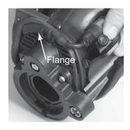
**NOTE:** To reduce snag hazards, stow the tube under the flange.
