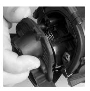
**NOTE:** Be careful not to lose or damage the exhalation valve spring.
