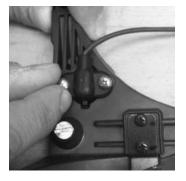
b. If screws are loose or missing replace both screws with MSA P/N 10034748-SP2. Use a screwdriver to ensure screws are hand-tight.
