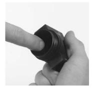
2. Apply Christo-Lube (P/N 604070) to both ends of the outer spring (P/N 10050620).
