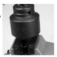
Installing the Pressure Relief Valve
