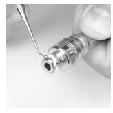
**NOTE:** Be careful not to damage the o-ring sealing surfaces.
