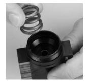
Removing the Seat and Seat O-Rings
