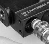
4. Install the high pressure gauge hose into the high pressure gauge port.
