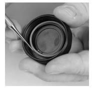
**NOTE:** Be careful not to damage the o-ring sealing surfaces.
