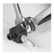
Screw the second stage hose onto the first stage intermediate pressure hose. Use the inch pound torque wrench and 3/4" crowfoot to tighten the threaded connection to 125 ± 5 in lbs.
