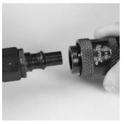
2. Connect test manifold assembly to first stage intermediate pressure hose.
