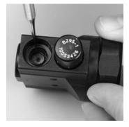
**NOTE:** Do not lubricate the filter o-ring.
