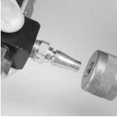
Connecting the Test Manifold Assembly, Quick-Connect Hoses
