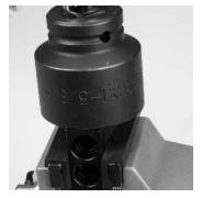
3. Use the o-ring removal tool to remove the cap o-ring.
