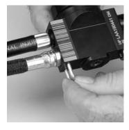
2. Pull the hose firmly to remove it from the regulator body.
