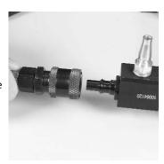
3. Disconnect the test manifold assembly from the first stage intermediate pressure hose.
