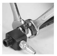
3. Screw the second stage hose onto test manifold assembly until tight.
