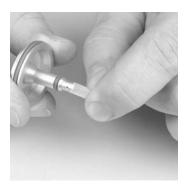
9. Install the piston into the regulator body.
