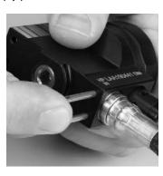
Installing the High Pressure Control Module Hose
