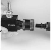
Connect the second stage hose to test manifold assembly.
