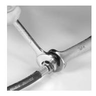
2. Screw the test manifold assembly onto first stage intermediate pressure hose until tight.
