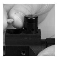
2. Install the filter o-ring into port and seat it against the filter.
