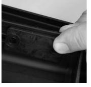
4. Remove residual thread-locking material from the bolts and mounting bracket threads.
