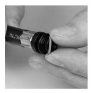
3. Install the intermediate pressure hose into the intermediate pressure port.
