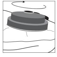
Lift edges of protective cover openings over cartridge bases and seal with tape.
