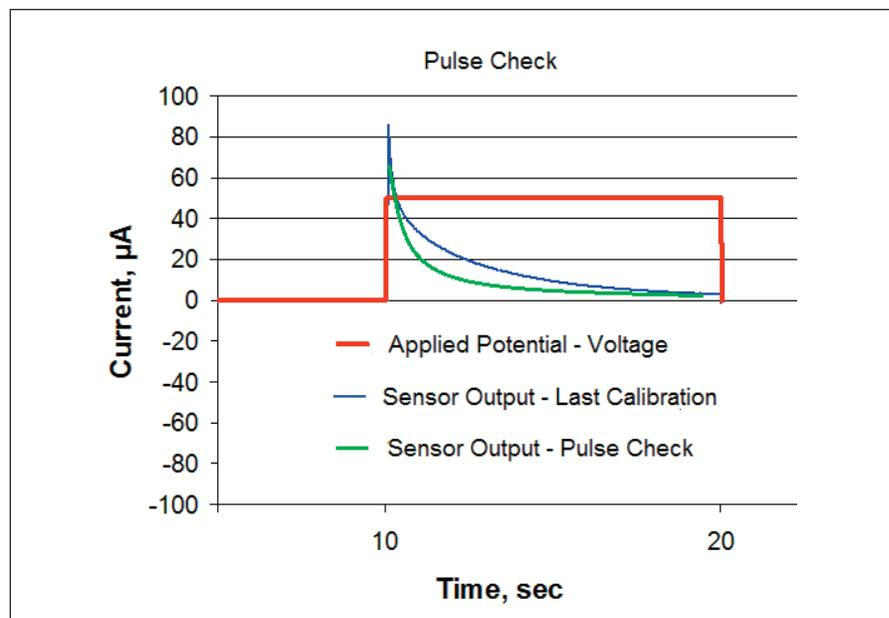
If a difference is measured in sensor response within acceptable range, correction can be applied to measured output to adjust the sensor for accuracy. Adjustment is possible due to ASICs used in MSA's XCell Sensors. If the output signal has drifted outside acceptable range, the instrument will notify the user that calibration is necessary.
