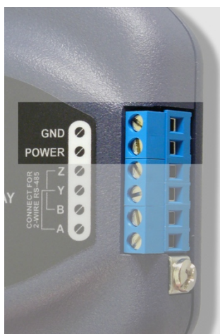
Figure 1: Terminal Block Power Supply Connections
