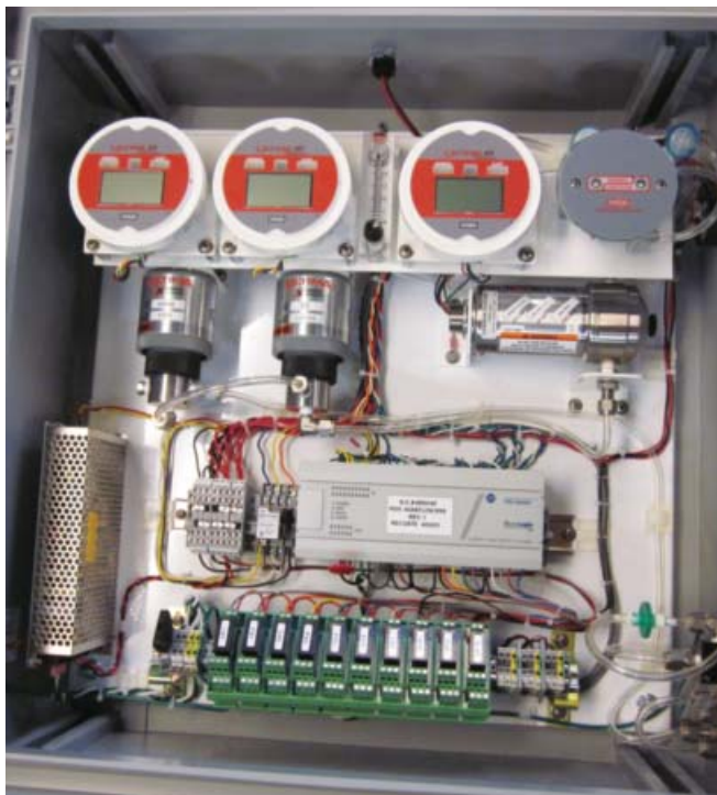
TriGas System for wet well monitoring in wastewater applications.
