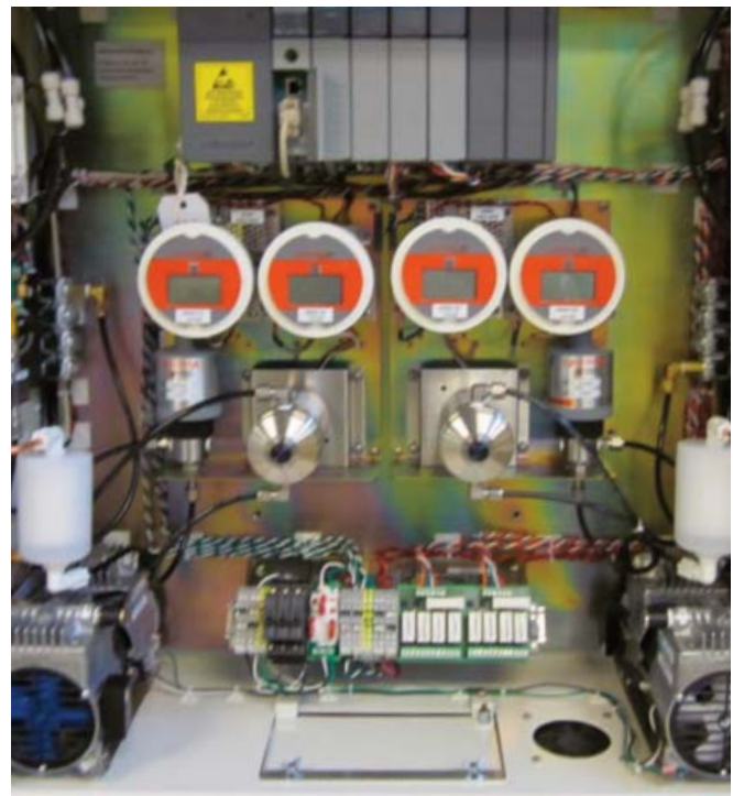
Multigard Gas Monitor with custom flow scheme and sensor options. Can sample up to 32 points.
