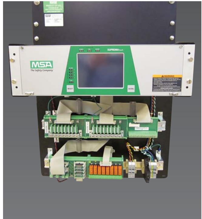
Suprema Controller with additional relays and custom configuration.
