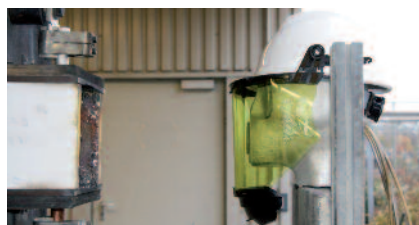
MSA vlamboogset vóór "boog-in-box-beproeving" 7 kA
