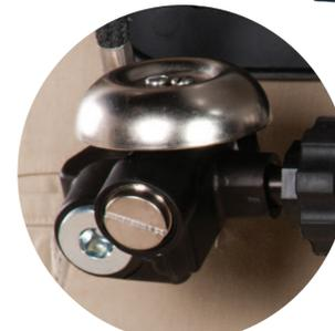
**Crack bypass valve** slowly to bleed off pressure until gauge needle drops below: 550 psig for 2216 Air Masks or 1125 psig for 4500 Air Masks. The alarm will sound. The alarm must continue to sound until pressure is less than 200 psig. Close bypass fully.
