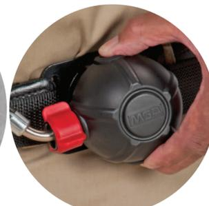
Close cylinder valve fully. Open bypass to **release system pressure**. Close bypass. Stow regulator with red bypass knob pointing to the right in STAND-BY belt mount.
