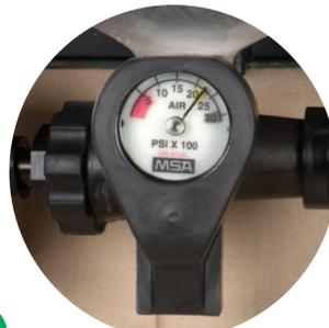
**3** Close cylinder valve and watch **pressure gauge**. If needle drops more than 100 psig in 10 seconds, there is a leak. Do not use the apparatus until the leak is found and corrected.
