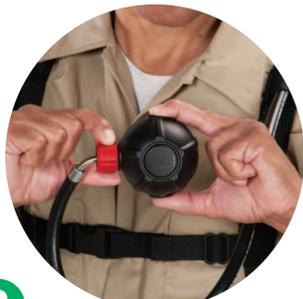
**2** Grasp mask-mounted regulator and push top release buttons. Check that **red bypass knob** is fully closed (clockwise).
