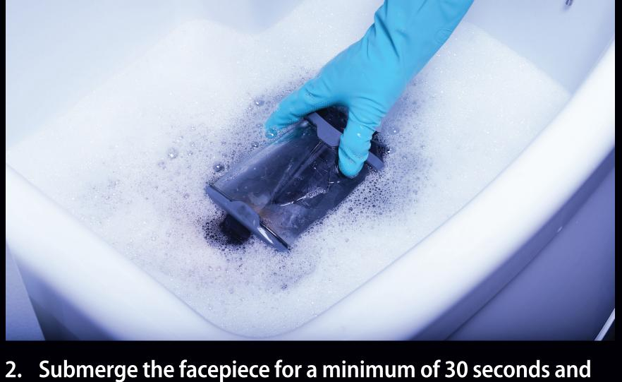
2. Submerge the facepiece for a minimum of 30 seconds and make sure the cleaning solution enters all areas of the mask.
