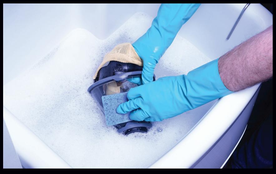
3. Scrub the facepiece inside and out with a soft, non-abrasive sponge or soft brush to make sure all contamination has been removed.
