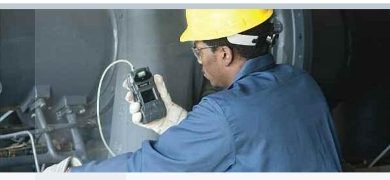
Oxygen deficiency or the presence of combustible gases is typical in gas storage areas and during oil drilling or gas treatment operations. MSA offers a full line of portable gas detection instruments providing early warning where there is a risk of explosion or exposure to toxic gas.
