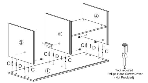
**Step 2:** Fix the screws from Part C onto board (10), and put Part D into the corresponding position (as per below diagram). Attach board (4) & (5) to board (10), and then fix the round screws from Part C with a screwdriver. Ensure all parts align.
