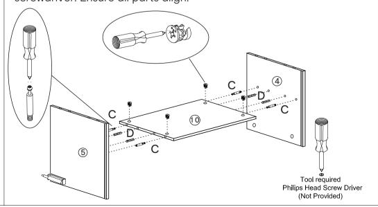
**Step 4:** Slide board  $\bigcirc$  into the corresponding position (as per below diagram). Ensure it is fully fitted in the grooves.
