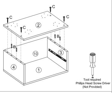
**Step 2:** Slide board ① into the corresponding position (as per below diagram). Ensure it is fully fitted in the groove.
