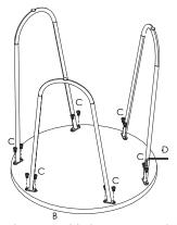
Step 3: Fasten all screws firmly, assembly is now complete.
