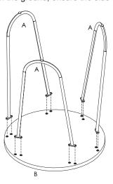
Step 2: Use screws (Part C) to fasten metal legs (Part A) to the board (Part B)
