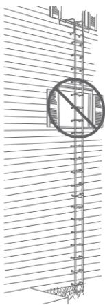
Do not use from a third floor window directly above a first or second floor window.
