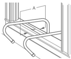
**DIMENSION A:** The windowsill width should be between a minimum of 6" (15 cm) and a maximum of 13" (33 cm).
