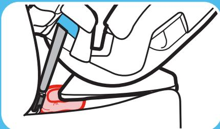
**Note:** For easier tightening, you may need to pull the tail of the lower anchor strap through the belt path as shown.
