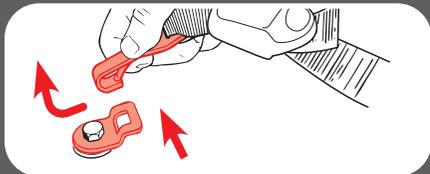
Press in on the hook's spring. Push tether hook in, then lift up and pull away from tether anchor.
