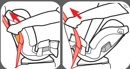
**Note:** With the vehicle seat belt in this locking mode, all the tension is upwards in the shoulder belt. This may start to tilt your car seat sideways. If this happens, use a locking clip instead of switching the retractor. See Sliding Latch Plate and ELR Retractor.
