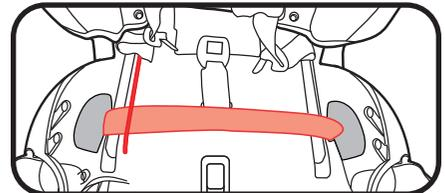
**Rear-Facing:** Make sure the lower anchor strap is in front of the buckle strap, is flat, and is not twisted.
