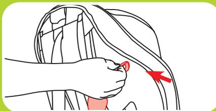
**6. Connect Lower Anchor Connectors to Vehicle's Lower Anchors**
