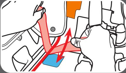
**3. Pull Lower Anchor Connectors Out of the Belt Path Openings into the Center of the Car Seat**
