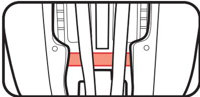
**Forward-Facing:** Make sure the lower anchor strap is routed behind the harness strap, is flat, and is not twisted.
