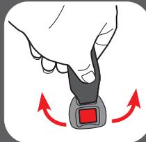
**WARNING!** Inspect and clean buckle from time to time to remove any objects or debris that could prevent latching.
