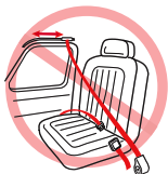
Lap Belt with Motorized Shoulder Belt
