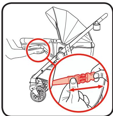
4. From the bottom of the seat, disconnect buckle on the foot end. **ALWAYS** release the webbing strap buckle to lower the foot end of the toddler seat before placing child in the bassinet.
