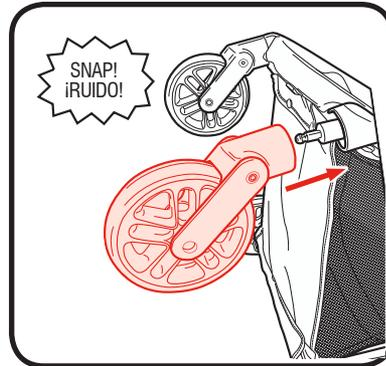
2. **CHECK** that wheels are securely attached by pulling on wheel assembly.
