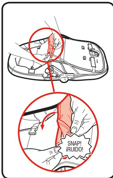
7. Snap side snaps around the two seat frame tubes.
