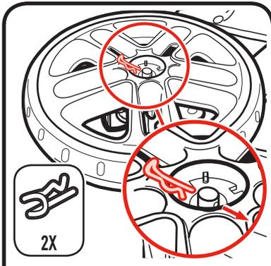
2. Push straight side of pin through axle hole. Pin will separate around the axle. Curved end of pin **MUST** face out as shown. Repeat on other end.
