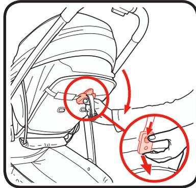
2. To raise the seat back, squeeze the button down, and pull up on both straps.
