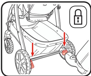
1. Push down on brake to lock brakes.
