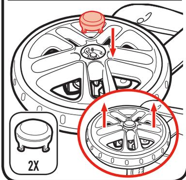
3. Attach hub cap as shown. **CHECK** that wheel is securely attached by pulling on wheel. Repeat on other side.
