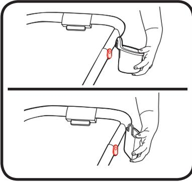
1. Line up opening in cup holder or phone holder with mount on stroller and press onto stroller tube.
