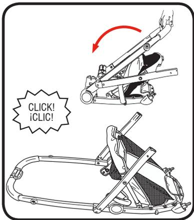
2. Lift handle of stroller up. **CHECK** that the stroller is completely latched open every time you open the stroller and before continuing with the rest of the assembly steps.
