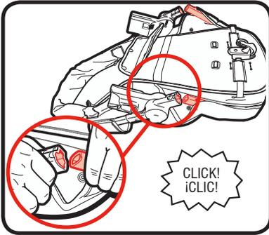
4. Attach seat frame tubes as shown.
