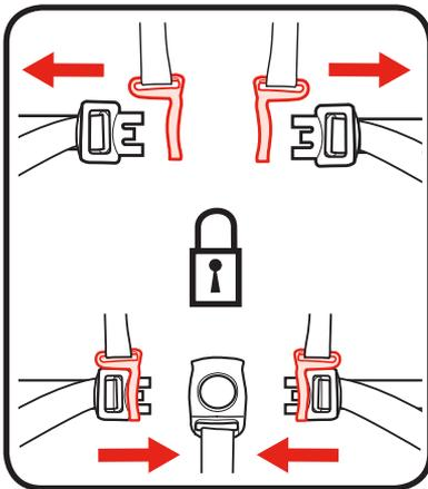
2. To close, slide shoulder strap connectors onto waist straps, and insert into buckle.
