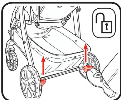
2. Lift up on brake to unlock brakes.
