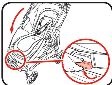
1. Pull bassinet handle then lower to place seat into toddler mode. Release handle to lock in place.
