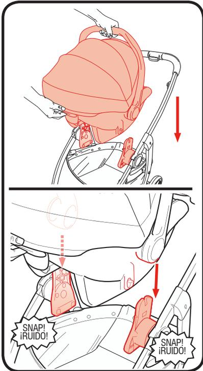
2. Insert car seat into stroller, and push down on car seat until the latches snap into the seat attachment mounts.
