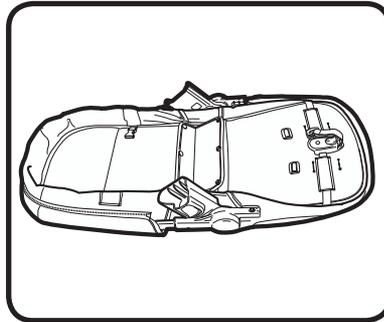
3. **MAKE SURE** the webbing does not block the mounts and frame tube connectors. Place webbing behind the mounts as shown.
