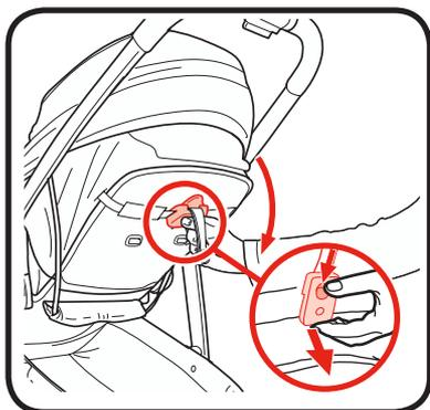
2. Recline the seat back by pushing button down, and pull down the seat.
