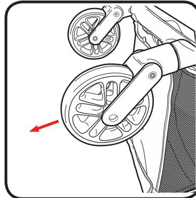
3. Remove front wheel by pushing button as shown.
