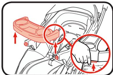
1. Remove child's tray by squeezing both buttons on tray and lift up.
