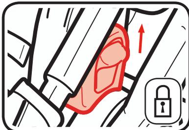
1. To attach seat, place seat on mounts as shown until they lock into place on both sides of the stroller. Seat may be placed on stroller in either direction.
