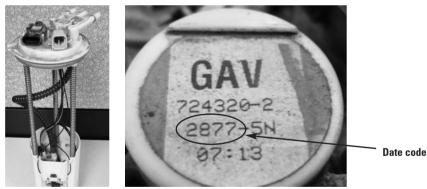
Fuel module is very aged and dirty. This module is an OEM part made by a competitor. The Delphi branded part is made by Delphi.
