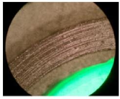
Contamination causing scratches on seal ring surface.
