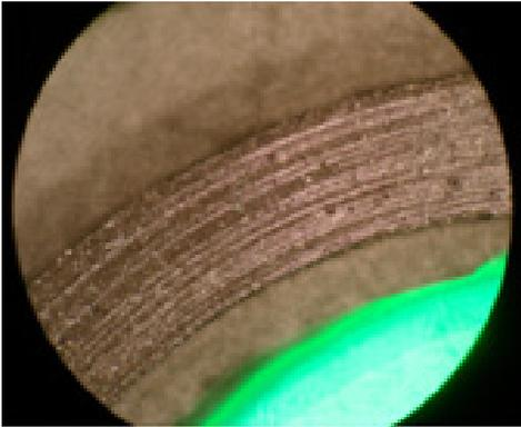
Contamination causing scratches on seal ring surface.
