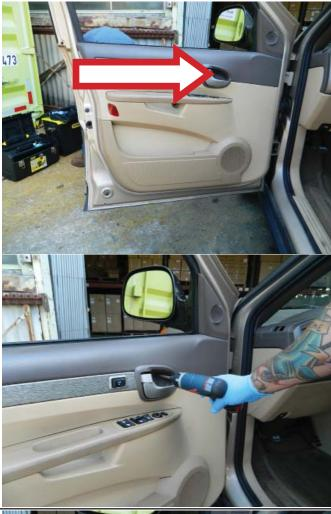
**STEP 2:** With the screw removed, you can use your non-marring pry tool to remove the trim.
