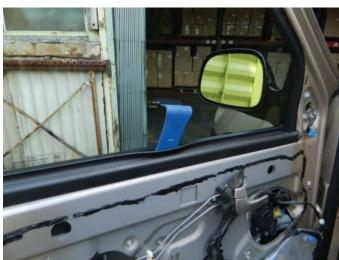
**STEP 12:** Remove the harness plug from the motor.
