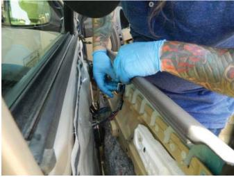
**STEP 6:** Install the door panel, taking care to feed the window switch harness through the hole in the panel.
