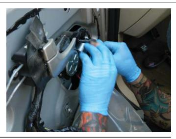
**STEP 3:** Lower the glass into the mounts by hand and tighten the 10mm bolts. You may need to temporarily attach the window switch to move the glass mounts to where you can access the bolts.
