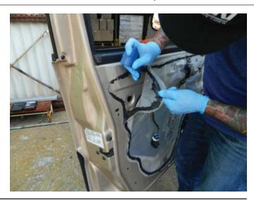
**STEP 10:** When removing the vapor barrier, it may be necessary to undo some harness clips to feed the harness through the barrier.
