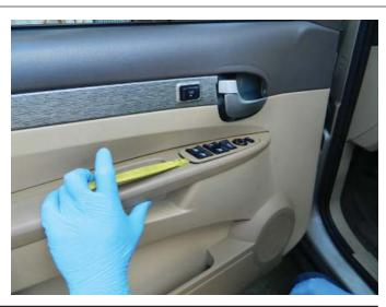
**STEP 4:** With the window switch removed, unplug the harness clips and set the switch aside.
