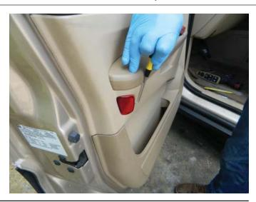
**STEP 6:** Using a 10mm socket, remove the bolt located behind the reflector and the bolt located under the arm rest.
