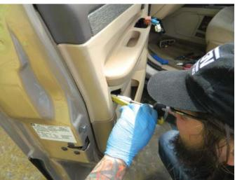
**STEP 8:** Reinstall the inner door handle trim with your Phillips head screw driver.
