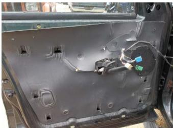
**STEP 9:** Temporarily install the power switch assembly to lower the window glass, exposing the screws attaching the window glass to the window regulator.
