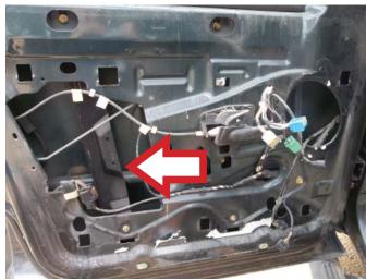
**STEP 2:** Using a 10mm socket and ratchet assembly, attach the five (5) window regulator attaching screws.
