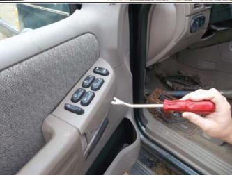
**STEP 3:** Disconnect the power switch assembly.
