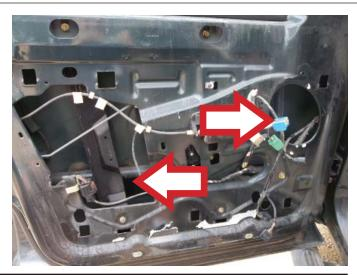
**STEP 5:** Once the door glass mounts are secure, attach the water vapor barrier.
