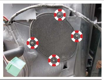
**STEP 8:** To attach the interior door trim panel, align the interior door trim panel retainers (which are part of the interior door trim panel) with the corresponding holes in the door and slide the interior trim panel in a downward motion. **NOTE:** Once the interior door trim panel is set in place, slide the interior door trim panel to align the interior door trim panel retaining screws into their original position.
