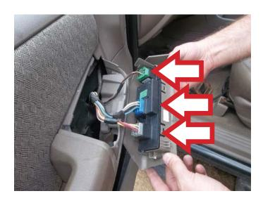
**STEP 11:** Attach the power switch assembly.
