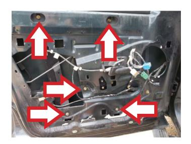
**STEP 13:** Remove the window regulator assembly through the main access hole.
