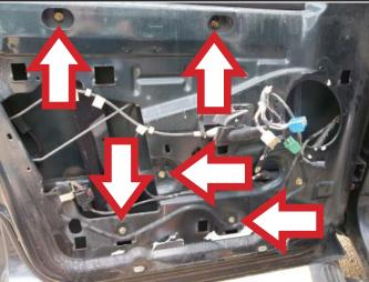
**STEP 3:** Connect the window lift motor connector.
