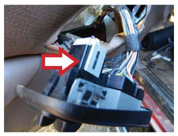
**STEP 3:** Once the interior door trim panel has been removed from the door, remove the master power switch assembly by lifting from the door trim panel and placing the master power switch assembly through the hole in the interior door trim panel.
