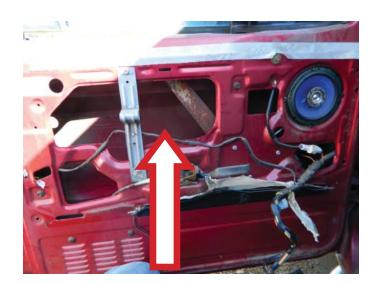
**STEP 9:** Remove the window regulator through the access hole.
