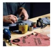
Water contamination and debris buildup are by far the biggest threats to your prized air impact wrench and other air tools. The common misconception is that if you regularly drain the air tank in your compressor, you are protecting your air tool from water damage, but this only prevents rust in the tank.
