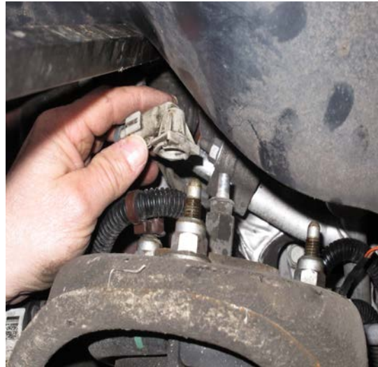
FIG 5, Rear Electrical Connection (detached)
