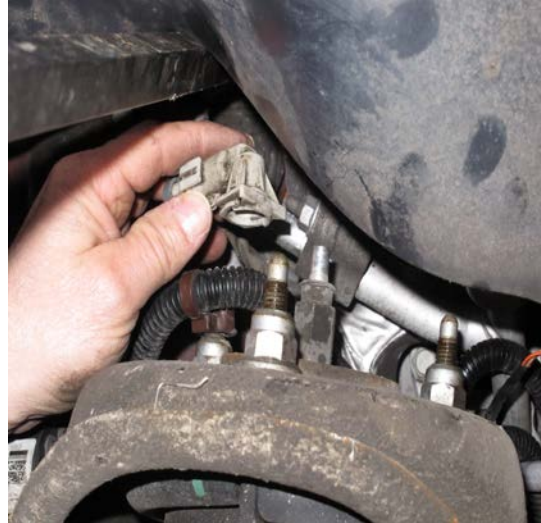
FIG 5, Rear Electrical Connection (detached)
