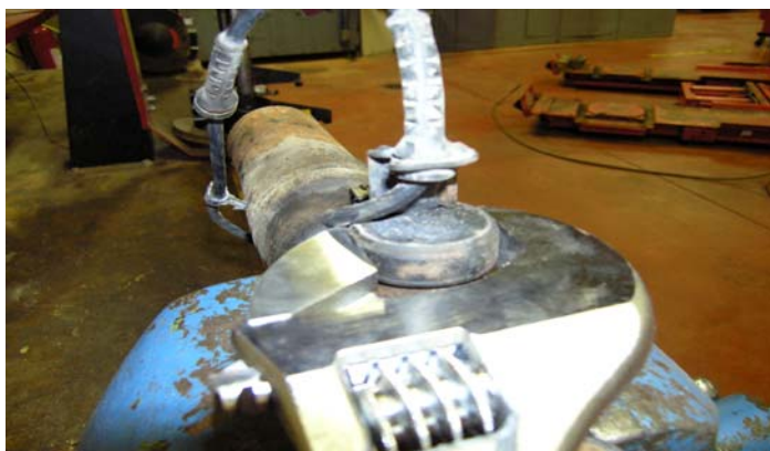
FIG 7, Rear Shock Solenoid Removed
