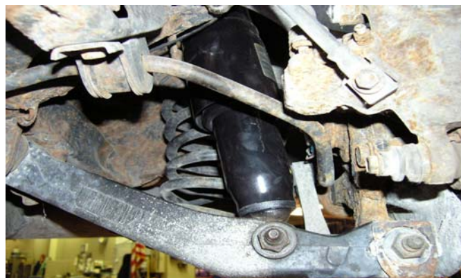
FIG 10, Rear Shock Installed Upper Portion Right Side
