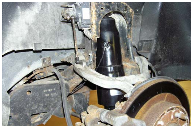
FIG 10, Rear Shock Installed Upper Portion Right Side
