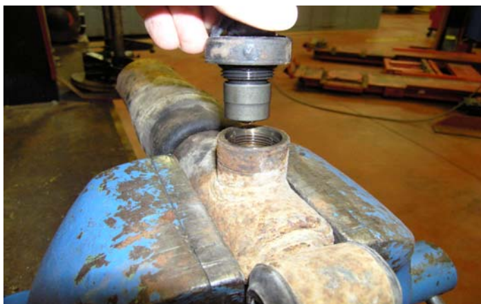
FIG 7, Rear Shock Solenoid Removed
