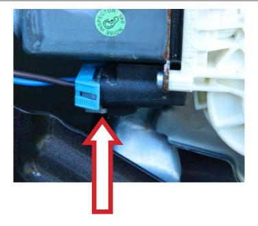
**STEP 4:** Temporarily install the power window switch. With the switch installed, raise the window regulator to meet up with the door glass. **NOTE:** It may be necessary to manually lower the door glass to align the mounting holes with the power window regulator.
