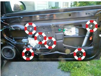
**STEP 13:** Remove the power window regulator mounting screws.
