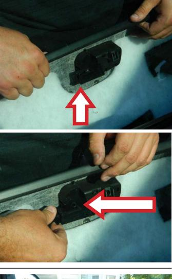
**STEP 11:** Place the interior door trim panel over top of the interior door weather strip. Once the door panel is secured on the interior door weather strip, align the interior door trim panel retainers with the corresponding holes and push into place.
