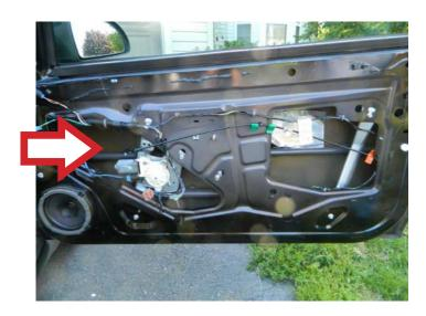
**STEP 1:** Install the window regulator through the access hole.
