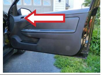
**STEP 3:** Using a trim panel removal tool, release the retaining clip attaching the door flag speaker assembly to the door.
