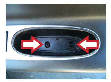
**STEP 12:** Attach the interior door trim panel to the door trim panel support bracket.
