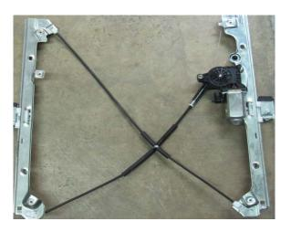
**STEP 2:** Install the left side track into the door.
