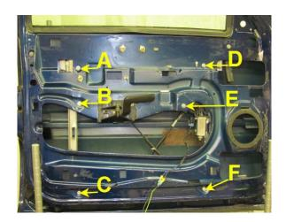
**STEP 9:** Lubricate the window run channels.
