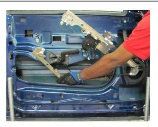
**STEP 3:** Install the right side track into the door.
