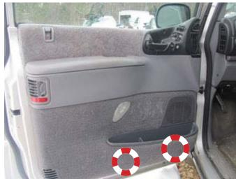
**STEP 2:** Remove the master power switch assembly screws from the bezel assembly.
