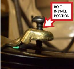
**STEP 6:** Install the left side track (side close to rear of vehicle) onto the door mounting slots – DO NOT TIGHTEN BOLTS!
