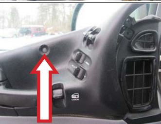
**STEP 3:** Gently lift the master power switch assembly up to expose the connectors on the back of the assembly. Disconnect the switch from the connectors.
