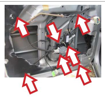
STEP 13a: Disconnect the window glass from the window regulator.
