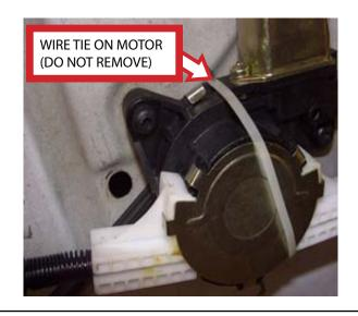
**STEP 2:** The regulator is supplied with the plastic window slides (mounts) already positioned for easy installation and glass attachment. Please double check for the presence of the two (2) clips as per the photograph.
