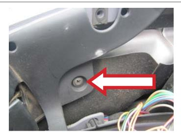
**STEP 5:** Using a trim panel removal tool, gently pry the door panel away from the door to release the door trim panel retaining clips. The retaining clips are located on the outer edge of the door trim panel and about every 4 inches around the door trim panel.
