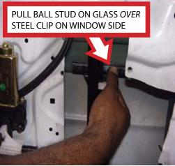
**STEP 11:** Place hand on the top of the window glass and pull the window hard to the left side door frame and into the window channel.
