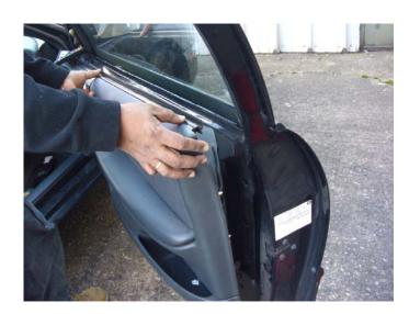
**STEP 10:** Install and connect the door cup assembly.
