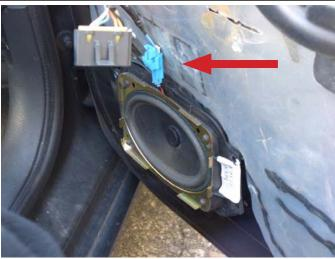
**STEP 6a:** Remove the four (4) screws that hold the door speaker into the door.
