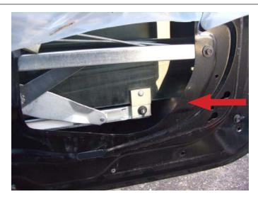
**STEP 8:** Push the window glass into the up position and use painter's tape, saddle cup assembly or wedge to hold the glass into the up position.
