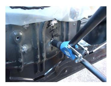
**STEP 4:** Install the power window regulator bolts, be sure NOT to overtighten the regulator bolts. Tighten bolts to 10 N.M or (89 inch pounds).
