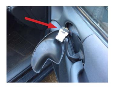
**STEP 3:** Remove mirror bezel assembly and three (3) Phillips head screws holding the door panel on.
