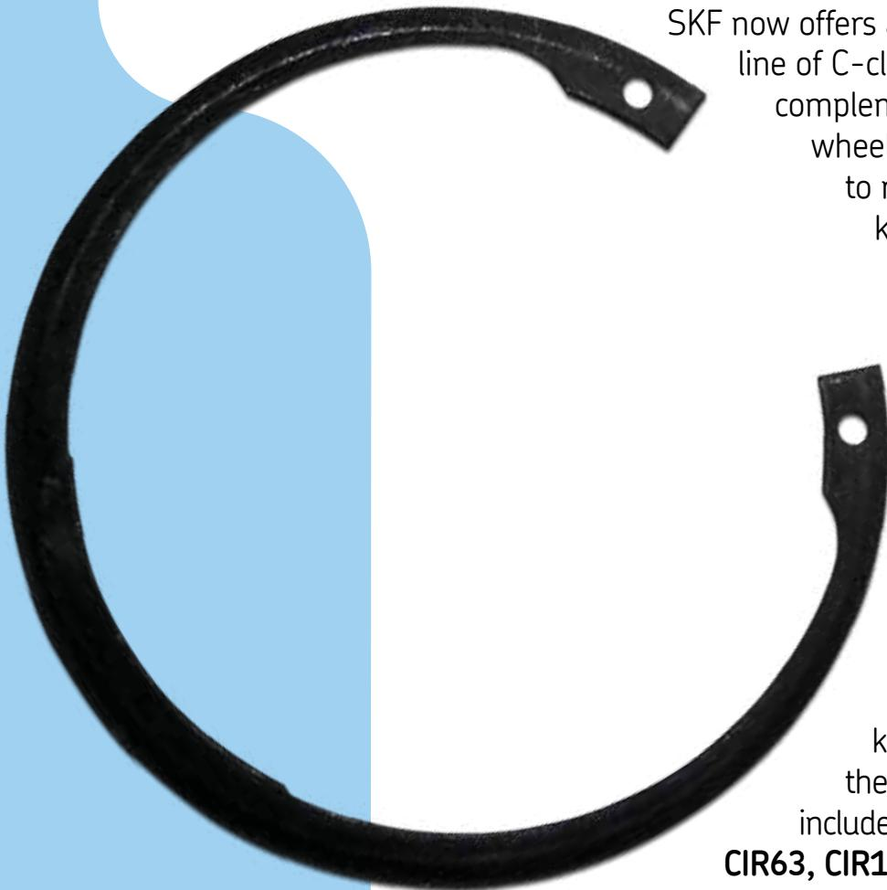
SKF now offers a comprehensive product line of C-clip retainers. SKF C-clips complement the Generation 1 wheel bearings, and are used to retain the bearing into the knuckle assembly.
